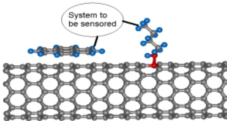
Fig. 8: Polymer-CNT composite system for a functionalized biosensor application. A polyethylene molecule is chemically bonded to a CNT and a pyrene molecular is adsorbed on the CNT through van der Waals interaction potential.
