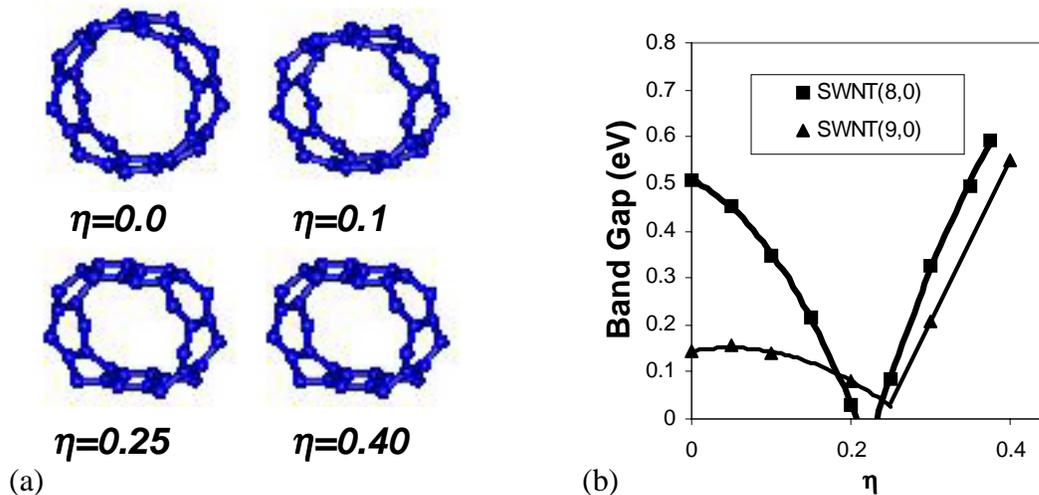
Fig.6 (a) The flattening of (9,0) carbon nanotube with four different degrees of deformation. (b) Energy band gap as a function of  $\eta$  for (8, 0) and (9, 0) SWNTs. The continuous lines are fitted through either quadratic or linear function.
