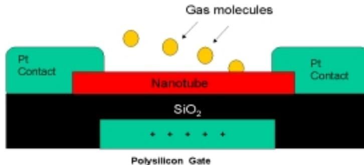
Fig.1 Schematic of a nanotube-based chemical sensor. The conducting properties of the nanotube change when chemicals in the surrounding environment bond to the tube. The absorbed molecules can act as dopants, shifting the Fermi energy of the nanotube. Similarly, the bonds formed between absorbed chemicals and the nanotube change the band-structure of the tube.
