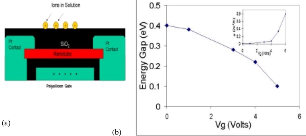
Fig.4 Schematic of an electrolyte insulator semiconductor (EIS) sensor, incorporating a nanotube sensing mechanism. A gate voltage  $V_g$  is applied to the semiconducting substrate and causes ions in the electrolyte to gather at the oxide surface. The conductance of the nanotube is modulated by the resulting electric field set up across the oxide. The strength of the electric field is used to identify the density and size of ions in the electrolyte.
