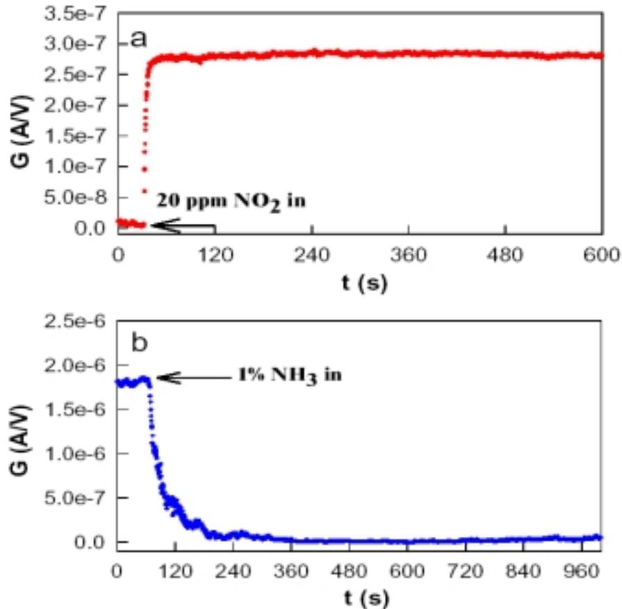
Fig. 2 Change of nanotube conductance when exposed to (a) NO<sub>2</sub> and (b) NH<sub>3</sub> gases.
