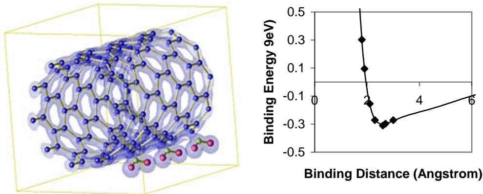
Fig 3 Left: Total valence electron charge density plot. The value of charge contour is  $0.0015 \text{ (e/\text{Å}^3)}$  showing the binding charge between the SWNT (10,0) and the NO<sub>2</sub> molecule. Three units are shown in this figure. Right: Binding energy curve for NO<sub>2</sub> interacting with (10,0) SWNT as a function of distance from NO<sub>2</sub> to the nanotube. The solid line curve is a fitting with universal binding curve.
